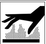
As for cylinder, crankcase, exhaust pipe, etc., during engine operation and after operation are extremely hot. Do not touch carelessly.
